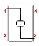
Pad 2 and Pad 4 are common and connected to the metal cover. They are not connected to the crystal.
